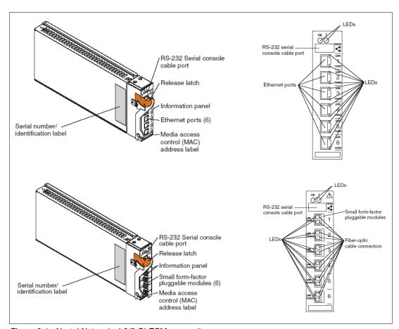
Figure 3-1 Nortel Networks L2/3 GbESM connections
